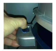
unlock the latches & remove the dust bin
