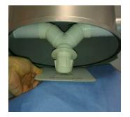
pull down and remove the old dust bag
